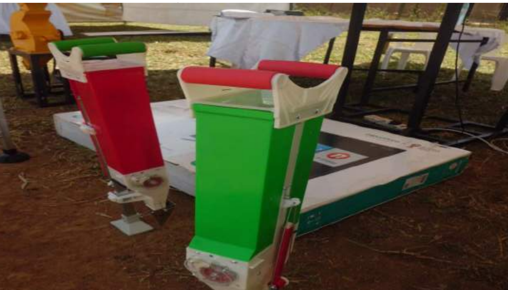
Plastic hand push seeders that are being used by farmers in Uganda for seeds planting. Photo Credit: Lominda Afedraru
